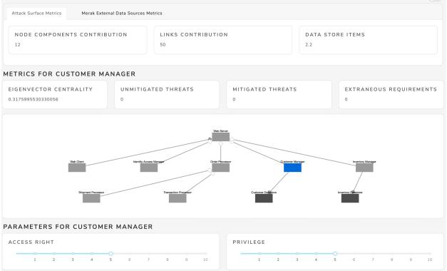
The transformations already show an improvement in the system's attack surface. Contributions from the components of the system towards the attack surface reduced from 18 to 12 and contributions of links towards the attack surface reduced from 65 to 50. With regards to centrality, the Web Server still has the highest centrality ranking of 0.64 followed by the Customer Manager at 0.32, Web Client at 0.26, and Customer Datastore at 0.13.
