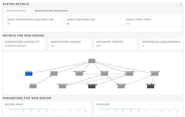
Alice notices that the attack surface increased from the baseline value of 18 to 20 for the components and from 65 to 66 for the links. The Customer Manager now has the highest centrality ranking at 0.42 followed by the Web Server at 0.19, Customer Datastore at 0.14, and Web Client at 0.07.
